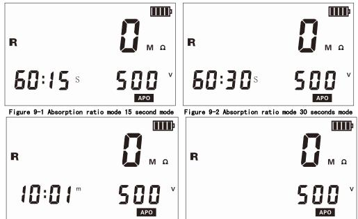
Figure 9-3 Polarization index mode
