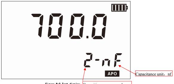
Figure 6-2 Test display Capacitive gear, second gear
