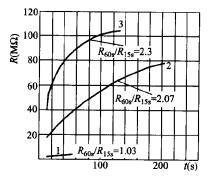
1—Hefor drying, 15 degree Celsius; 2-When the end of drying, 73.5 degree Celsius 3-After running 72h, and cooled to 27 degree Celsius
