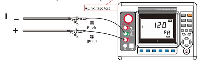
2. During the current test, the units of mA are shown in Figure 5-2, and the units of nA, uA, and pA are shown in Figure 5-1.
